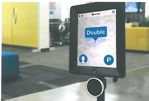
Double® 2 is there when you can't be. Double® 2 is the world's leading telepresence robot, providing a real, physical presence at work or school via a two-wheeled balancing robot with an attached iPad®. Weighing only 15 pounds, a user attaches an iPad to the Double unit then uses an iPad, iPhone® or web browser to control and drive the robot.
